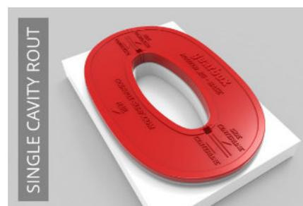
cavity first. Then finish off by moving the router in a clockwise direction around the perimeter of the jig. This will protect the outer edge of the cavity from debris flying around inside the cavity. Resulting cut is always a 1/16" offset from the jig.
